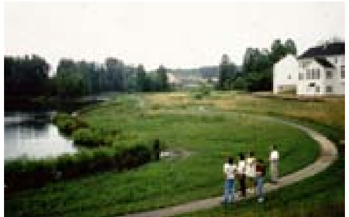
Figure M4.4: Vegetated buffer.
